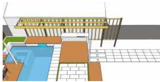
OVER VIEW OF FRAMING COMPONENTS FOR CANOPY.
